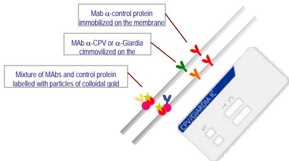
The device consists on a plastic casing with 4 windows:
